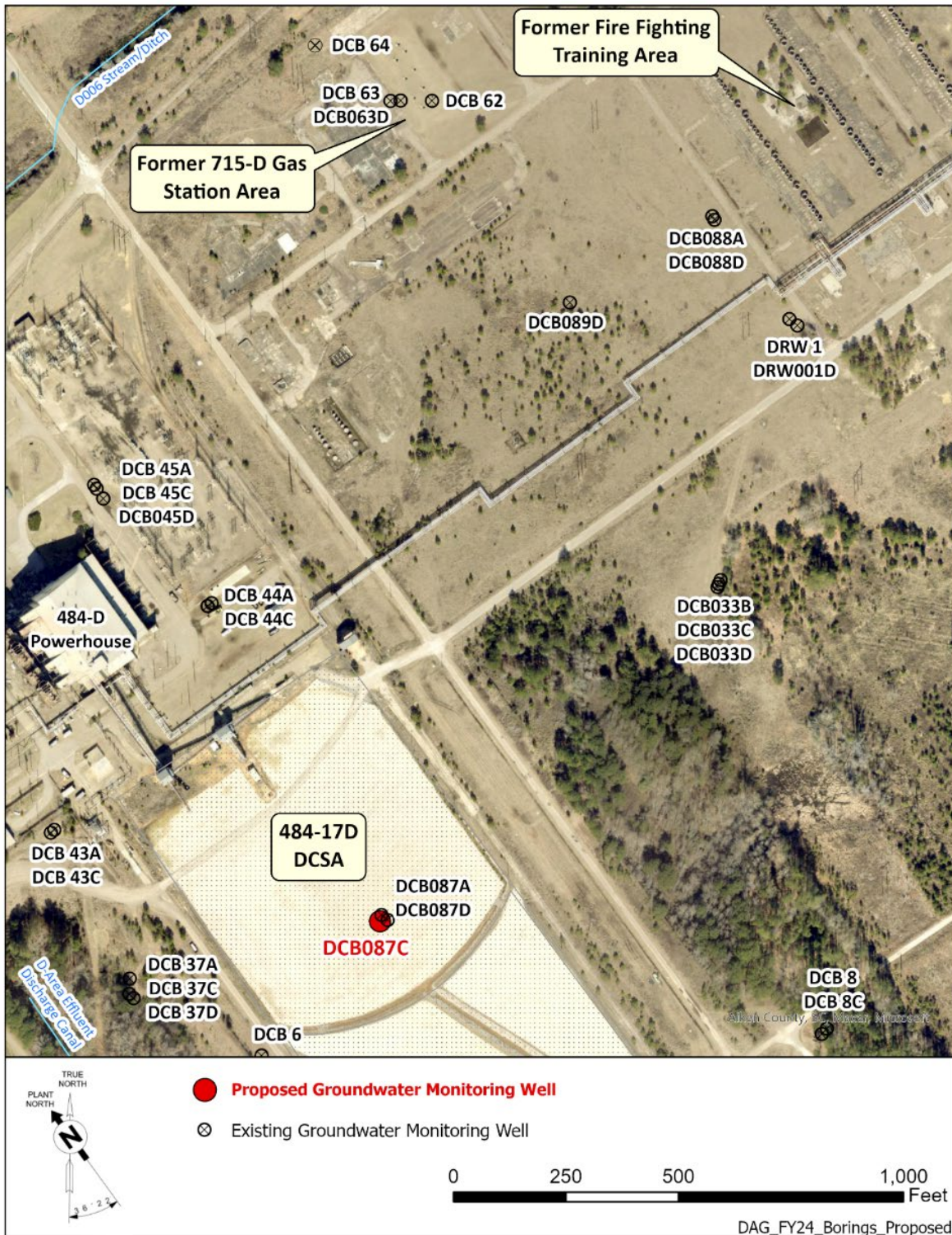
Figure 13. Proposed 484-17D DCSA Groundwater Monitoring Well Location
