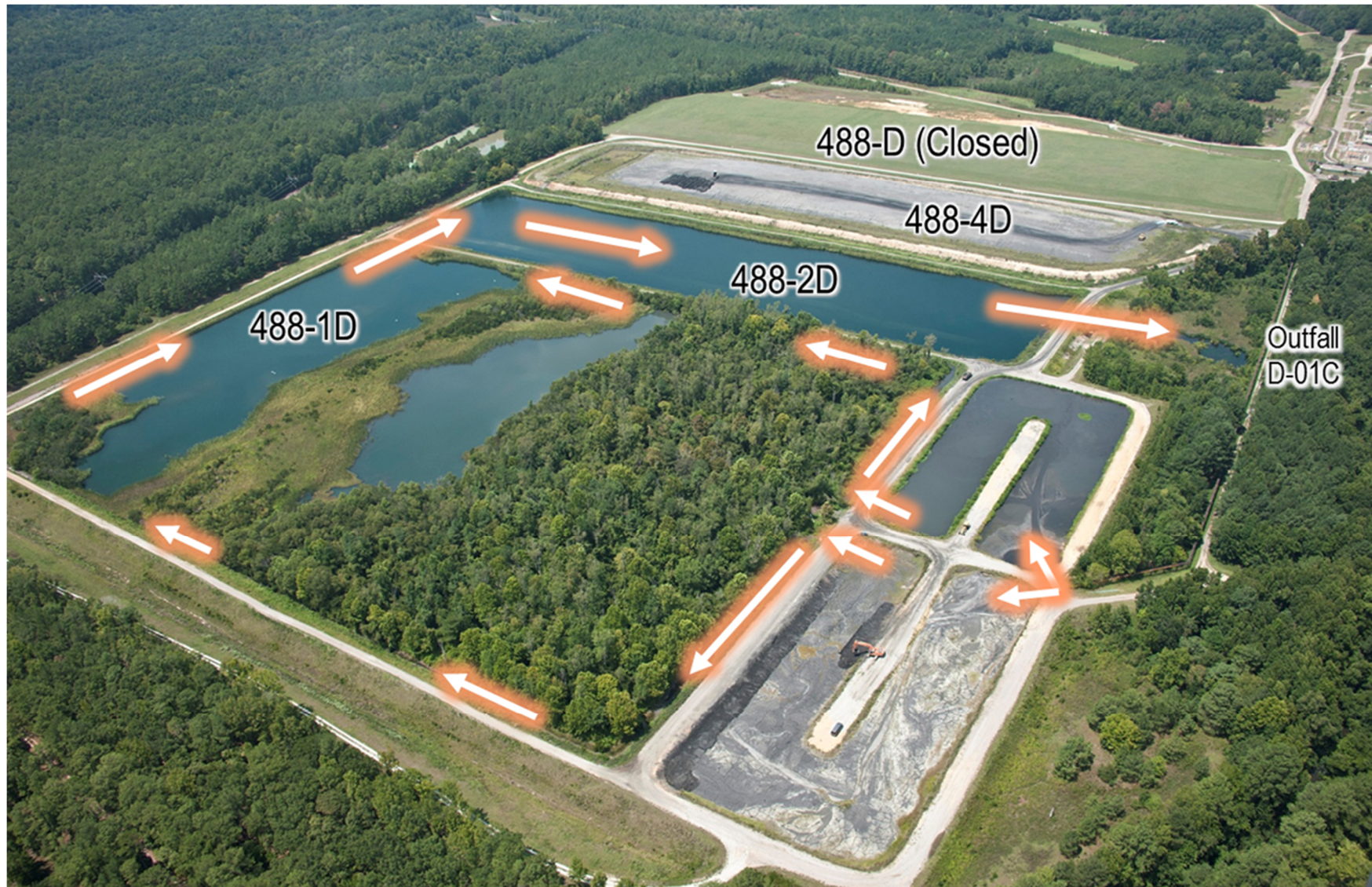
Figure 5. D-Area Ash Basins Waste Water Flow Pattern During Operations
