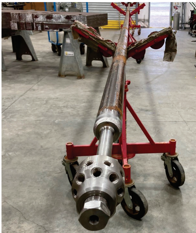
Figure 7: Tank 27F Hydrolancing Tool
