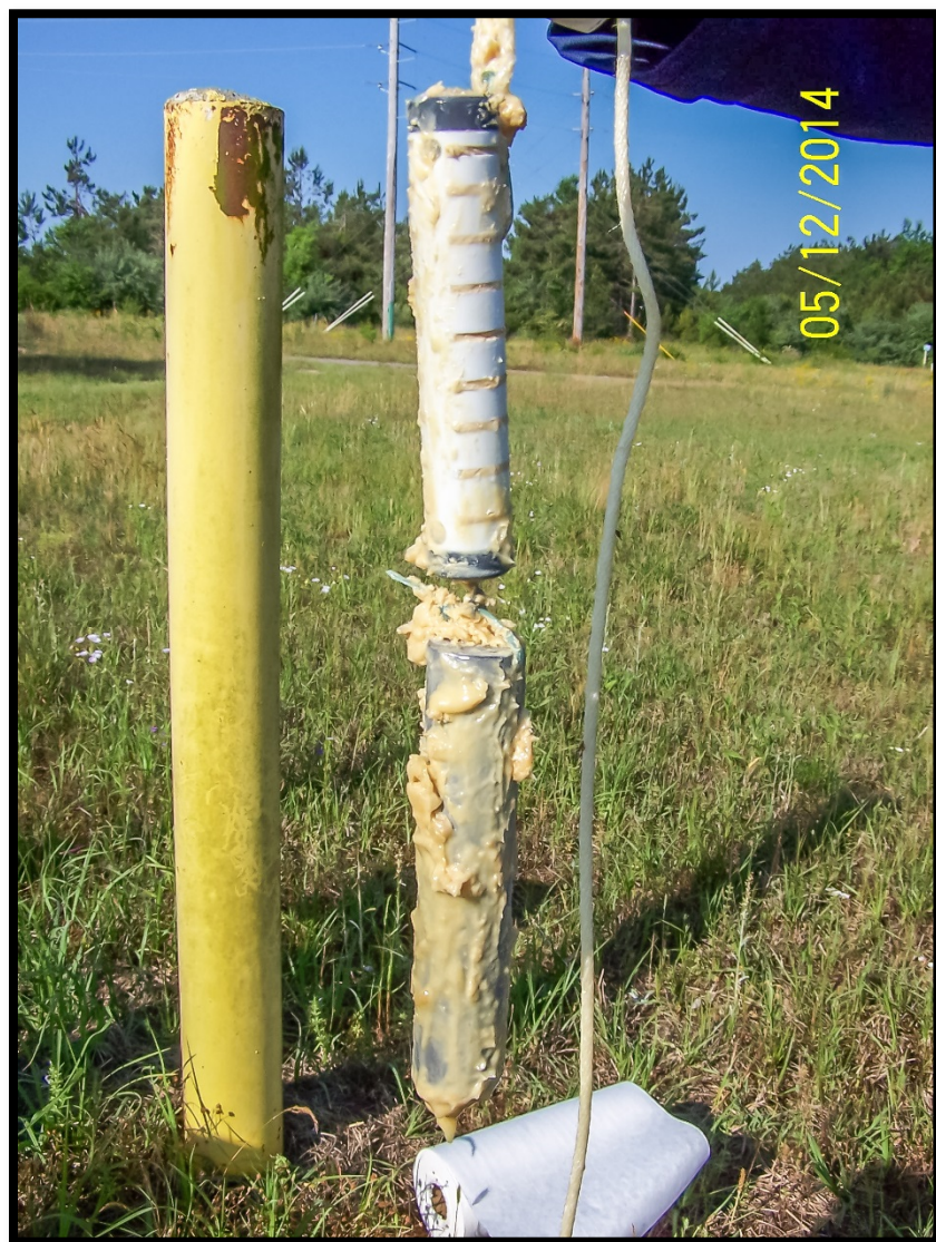
Figure 12. Photograph of BioTrap® from Injection Well PMW003DL
