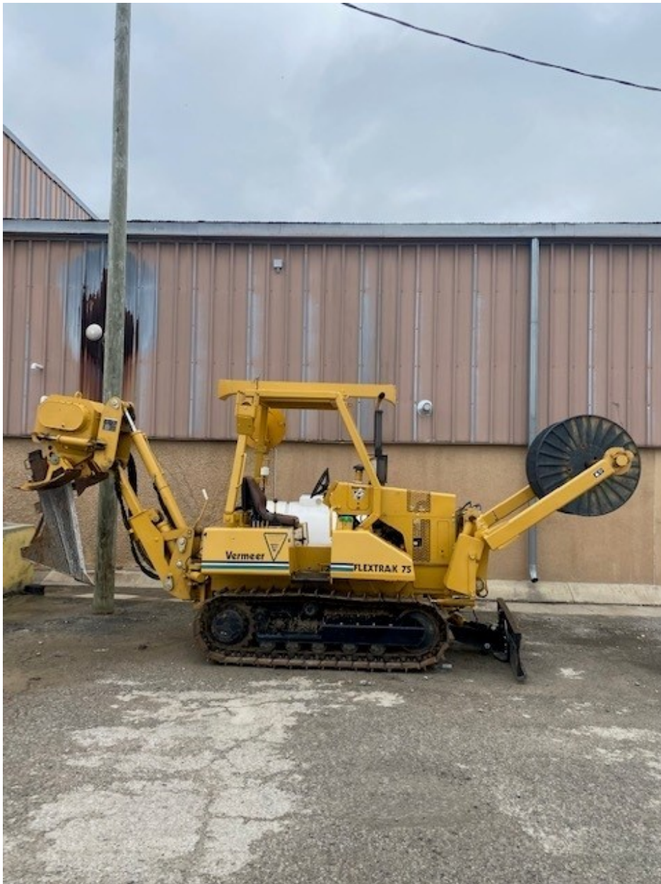
Figure 2. Bulldozer, mole plow, and cable reel.
