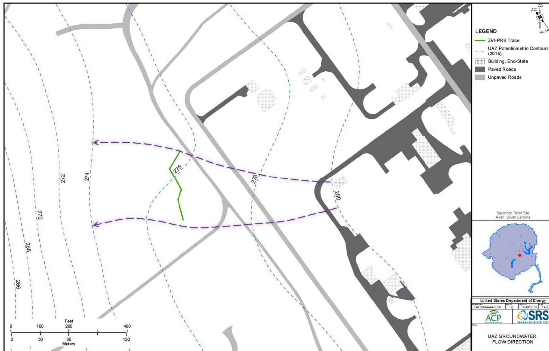
Figure 11. PAGW OU UAZ Groundwater Flow Direction and Potentiometric Surface
