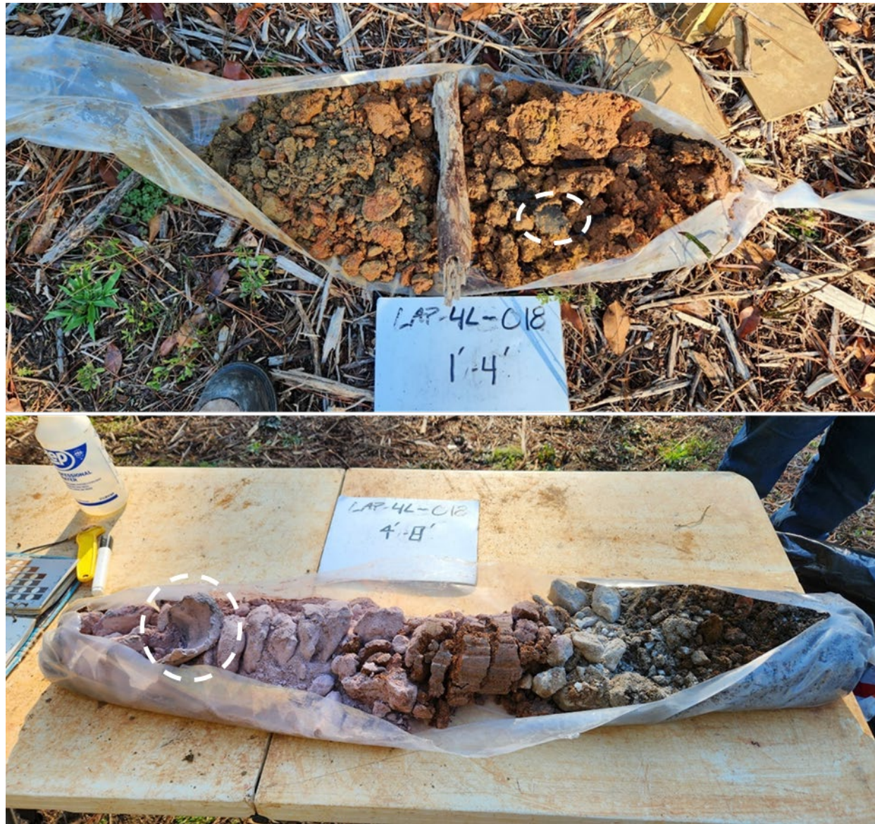
Figure 3-8. Photo of Asbestos-Containing Material Determined in Sampling Location LAP-4L-018
