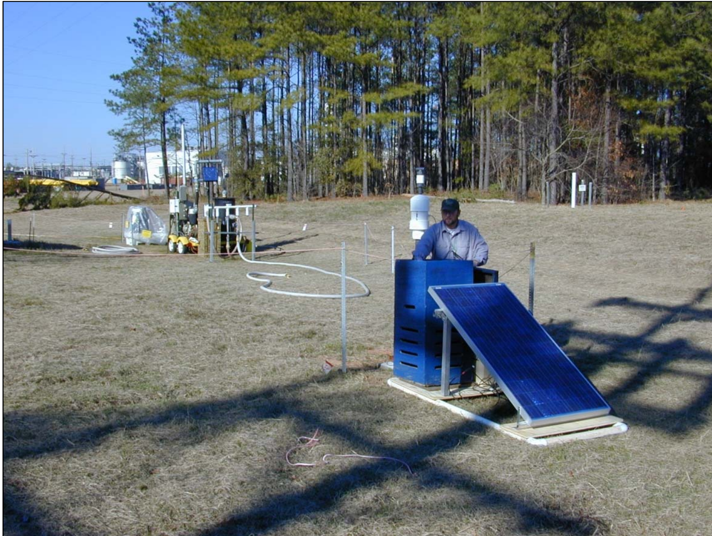
Figure M-5. Photograph of a MicroBlower™ Field Setup powered by a Solar Panel (2007)
