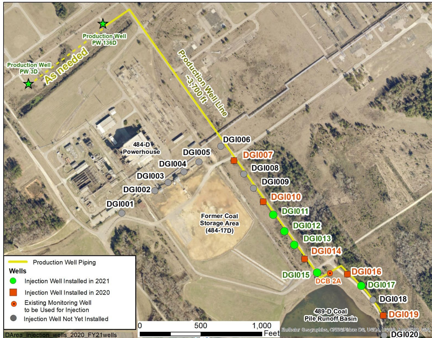
Figure 7. D-Area Injection Wells Installed and Production Well Piping
