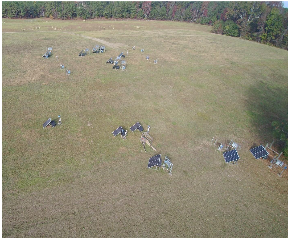
Figure 3. Aerial Photo of the ABRP MicroBlowers™ and BaroBalls™ at SRS (2022)
