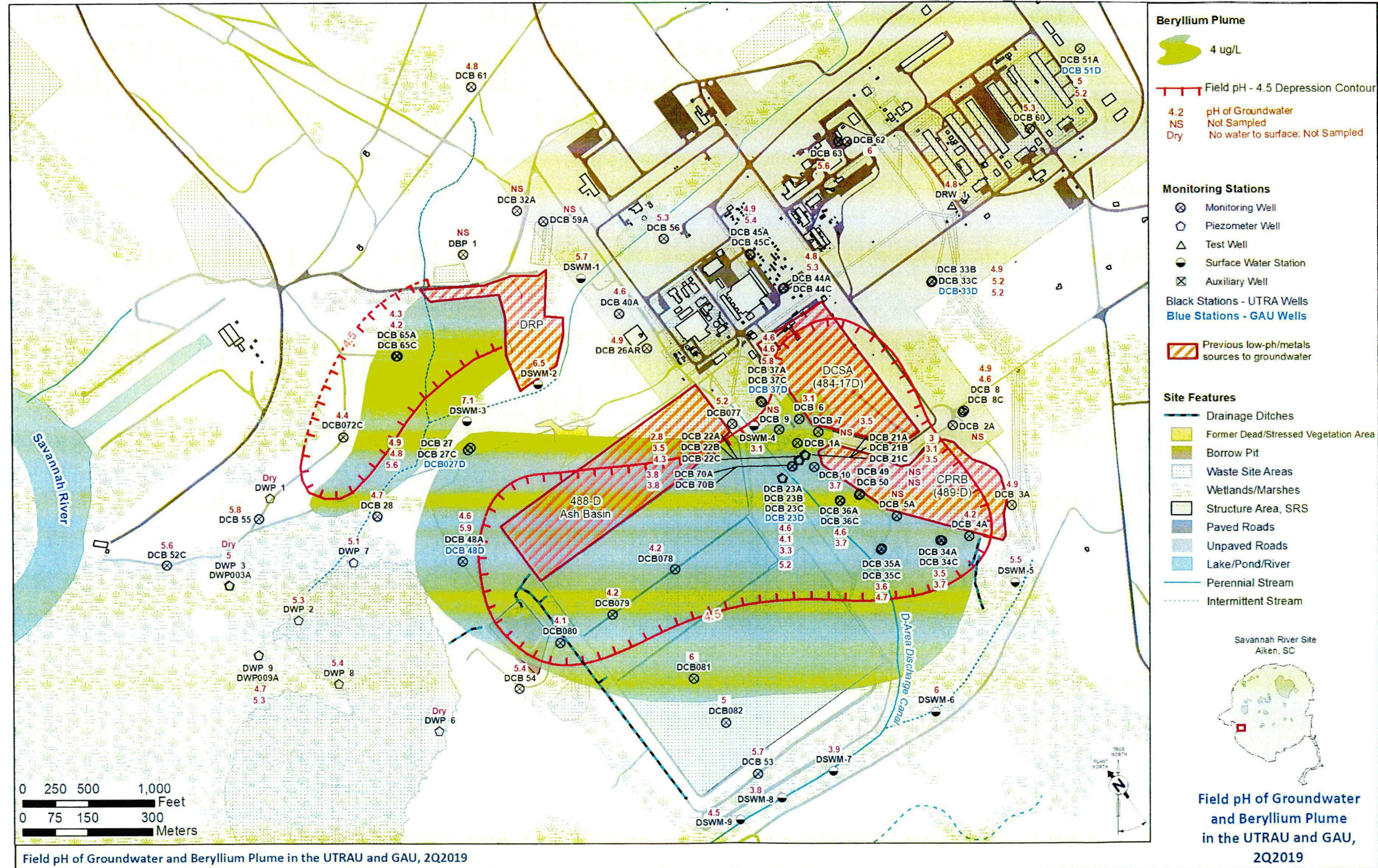
Figure 6. Field pH of Groundwater and Beryllium Plume in the UTRAU and GAU, 2Q2019
