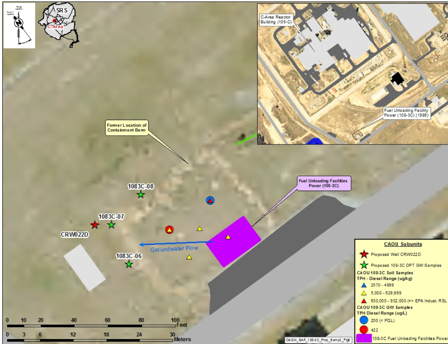
Figure 6. Fuel Unloading Facilities Power (108-3C) TPH and Proposed DPT and Well Locations
