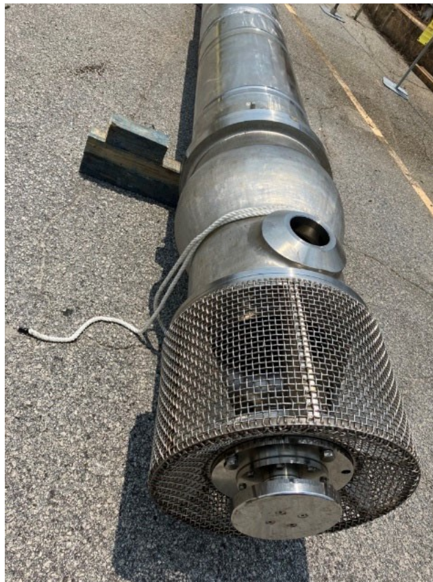
Figure 9 - Tank 15H Slurry Mixer Pump
