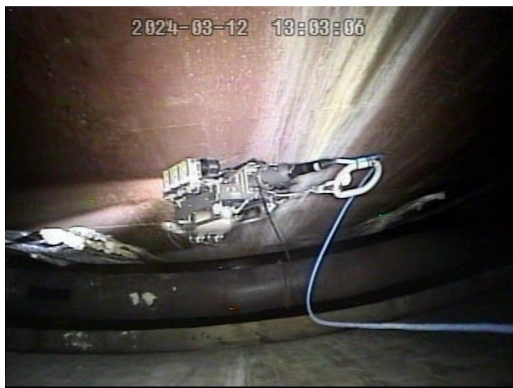
Figure 7 - Tank 10H Magnetic Crawler Below South Annulus Riser
