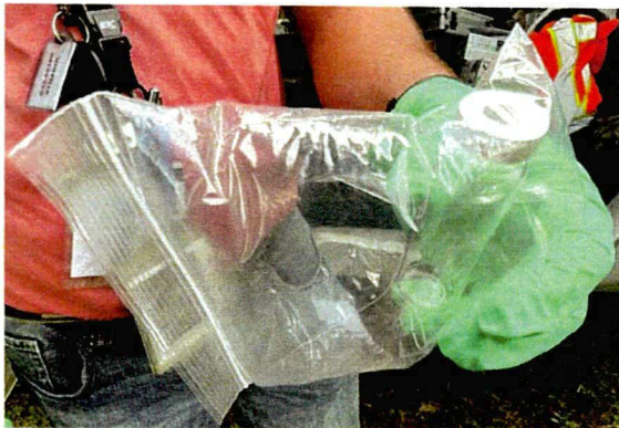
Soil vapor sample is now sealed
