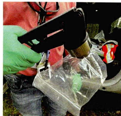
Seal the bag, put the cap on the vial, and crimp the cap through the bag
