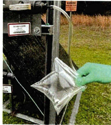
Insert tubing from MicroBlower™ or vacuum pump and purge three times
