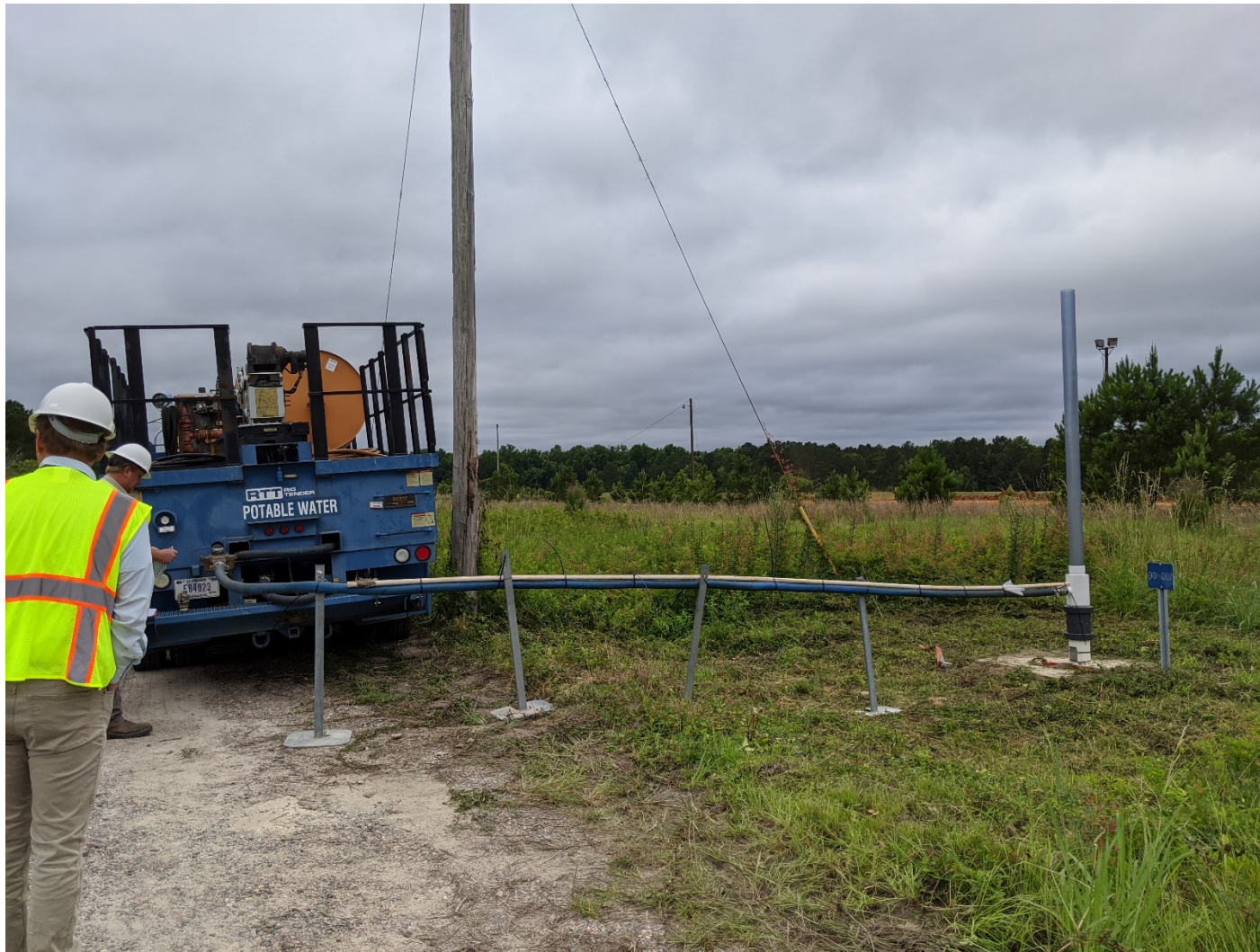
Figure 12. Slug Testing at Injection Well DGI007
