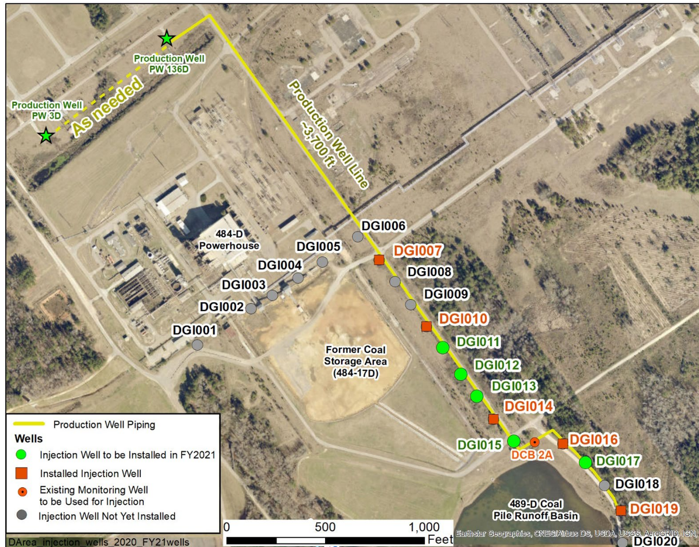
Figure 9. D-Area Injection Wells Installed and to be Installed in 2021
