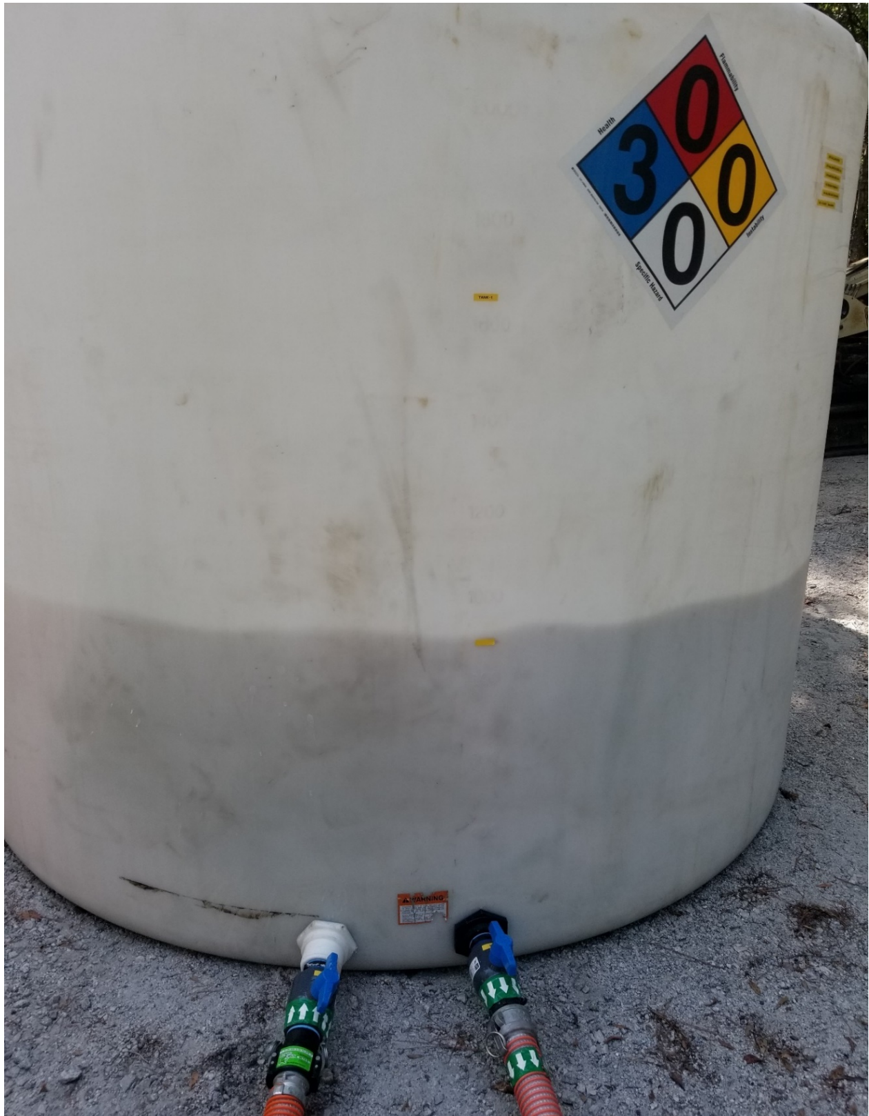
Figure 7. EOS Emulsified Oil Mixture Half-Batch Mixing
