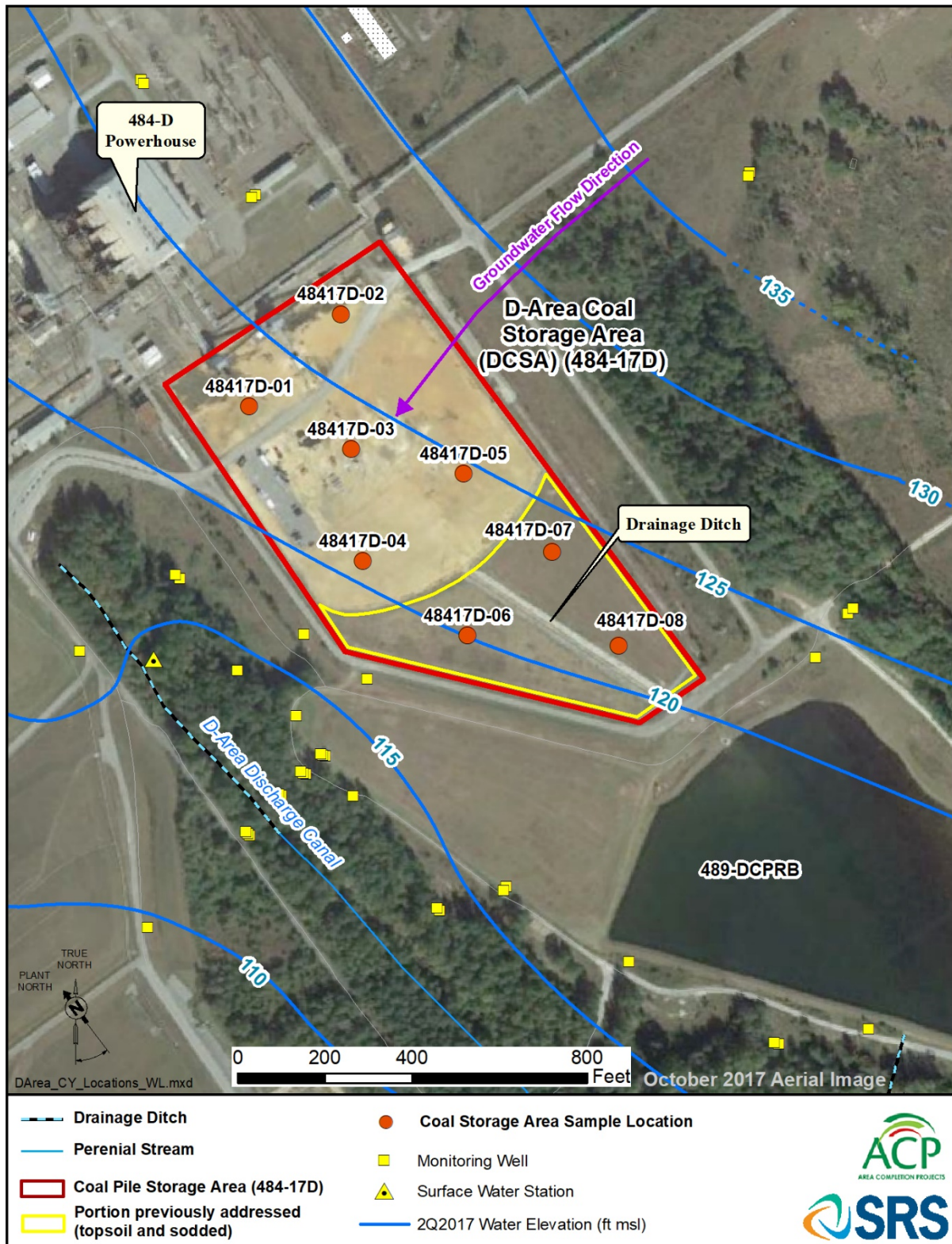
Figure 5. June 2018 Soil Sampling Locations within the DCSA
