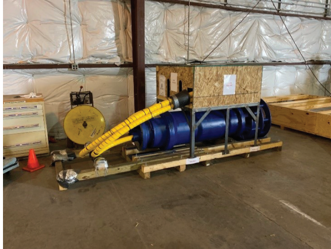
Figure 8: Tank 33F Enhanced Commercial Submersible Mixer Pump (ECSMP)
