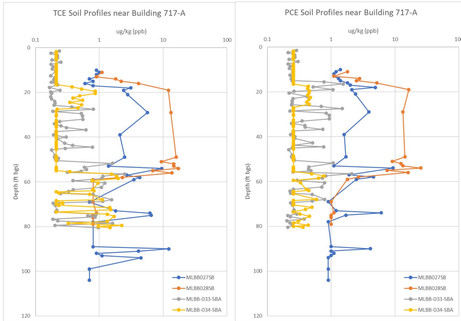
Figure E.8-23b. TCE and PCE Soil Profiles at Vertical and Angled Soil Borings near Building 717-A
