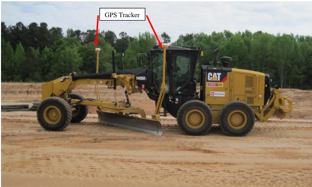
Photo 14. GPS Equipped Motor Grader (CAT 140M)
