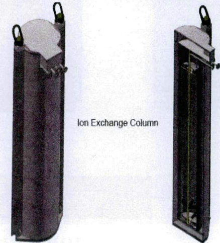
Shielded Ion Exchange Column (IXC)
